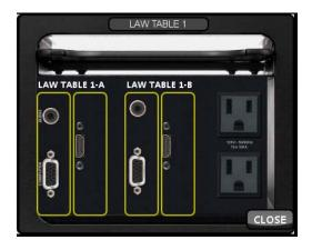
Table inputs include 2 HDMI and 2 VGA inputs at each of the Counsel Tables. Select any 2 of these inputs for use at the same time to be routed to the displays: VGA - VGA; HDMI - HDMI; VGA - HDMI; or HDMI - VGA.
