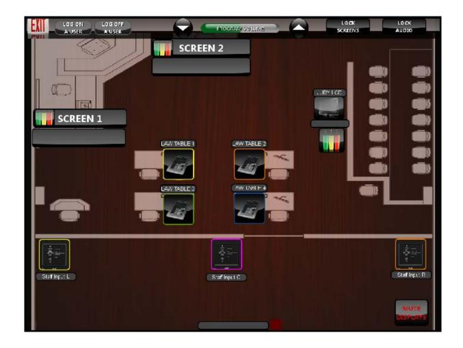
The Main Page is where the user selects the System input, and selects the screen or screens on which the input is to be displayed. This is also the page on which the user selects the screen on which to perform the Annotation and to be sent to the Record. In addition, this screen controls the audio input and output.
